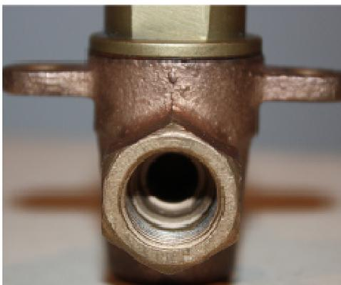
This photo shows the outlet of the valve with the plug turned to the open position. Bill Pancake told me that when Imperial originally manufactured these valves the bore through the valve body and plug was smaller than shown but that Aeronca increased the valve passage to 5/16". Bill said that sometimes you will come across a valve with a bore smaller than 5/16".
