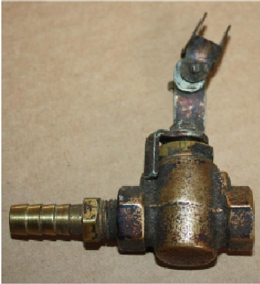
This is a photo of a fuel shutoff valve that was actually removed from a Champ. While it was a tapered plug brass valve somewhat similar to the two valves shown on the previous page, it is NOT an approved valve for use on certified planes such as the Champ or Chief. This was a standard plumbing valve typically sold in the local hardware store. The shaft on this valve was modified with a homemade universal joint to connect to the Champ fuel shutoff linkage.
