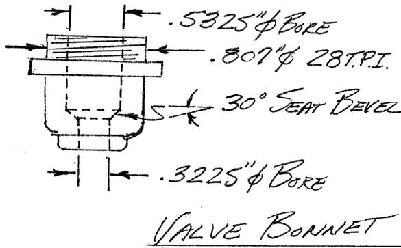
Measurements from old style valve with shaft packing as shown on page 2
