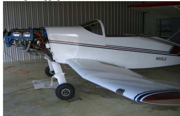
Aircraft partially disassembled for condition inspection
