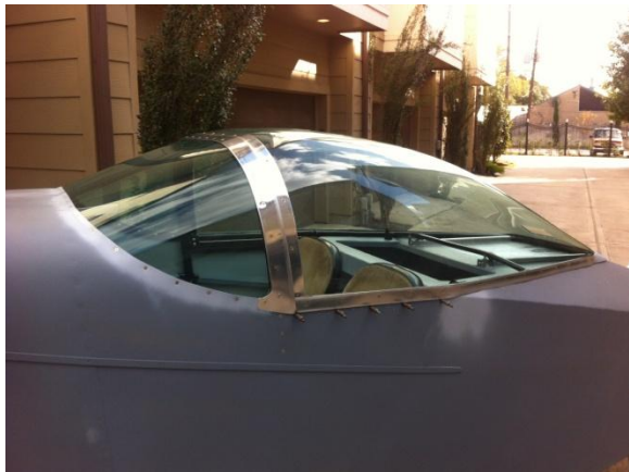
Gary Cotner's old canopy refitted on N118LW, glass was actually in immaculate shape, not bad for being 20+ years old.
