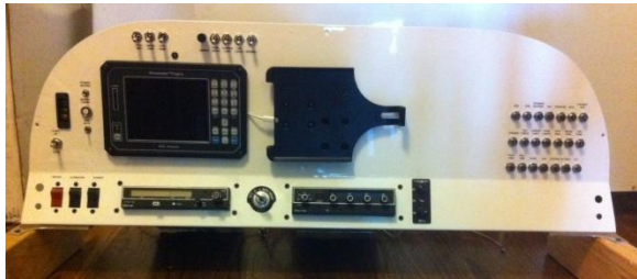
David Read’s old Enigma found its way to Houston for use in N118LW; mount next to the EFIS is for an iPad – Mini
