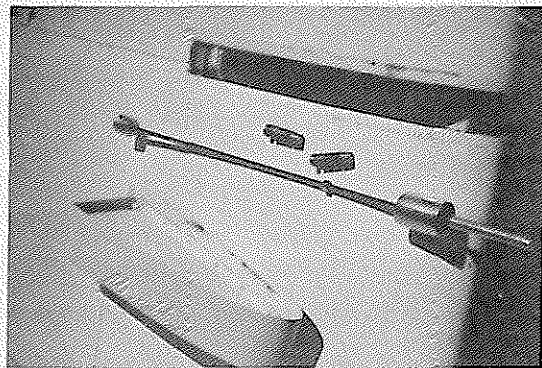
LU'S CW PIN EXTRACTOR TOOL AND CAP COVER →
